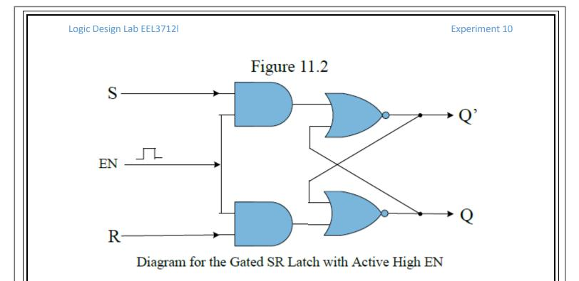
The truth table in Table 11.2 shows how the **EN** input controls when the latch can respond to the **S-R** inputs.
