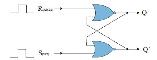
Figure 11.1 SR Latch with NOR gates
