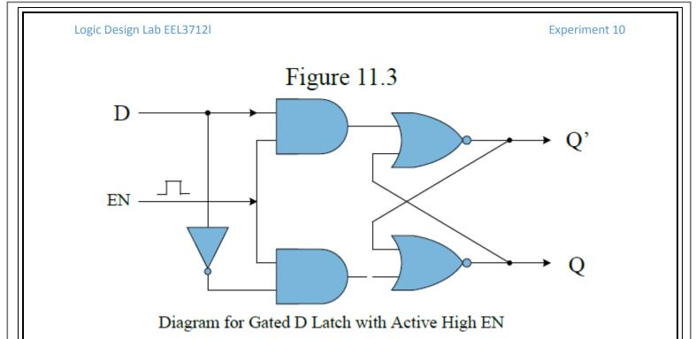
By examining the following truth table, we can see that a level-triggered **D FF** has a simple operation. The output **Q** simply follows the data input **D** when the enable input is activated. **Q** is latched when the enable is low. There is no invalid state in this latch.
